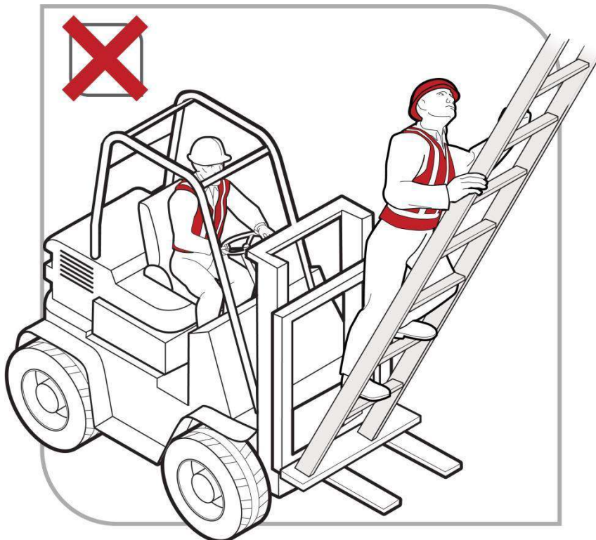
Figure 15 Unacceptable practice with ladder on forklift
