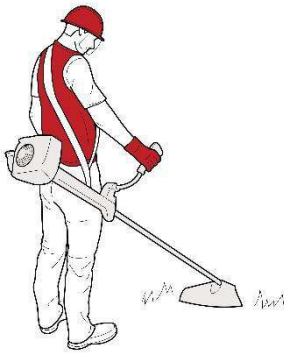
Figure 32 Weight supported by a harness; heaviest part of the brush cutter located behind the wrists
